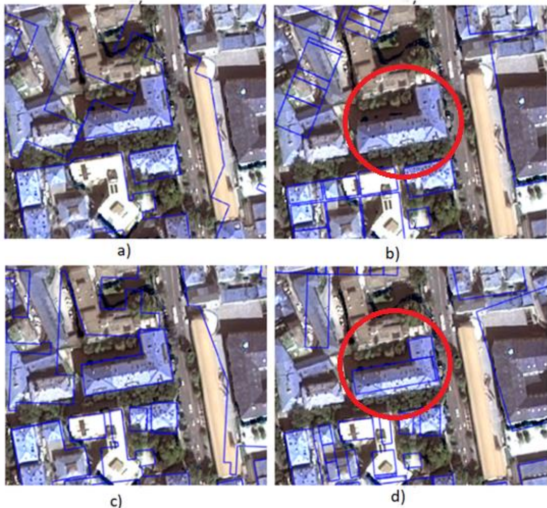
Figure 20: Figures a) and b) show initial building outline extraction and decomposition from building mask, c) and d) initial building outline extraction and decomposition from our building border detection.
