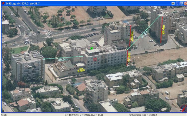
Figure 5. Height and distance measurements (Aeromap, 2006)
